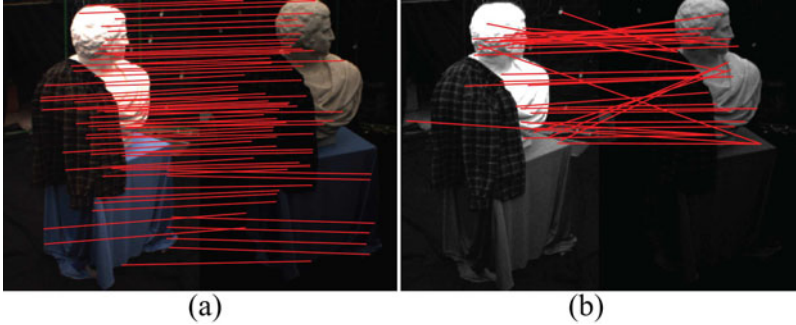
Fig. 4. Correspondence matching results: (a) our method and (b) SIFT-based method
